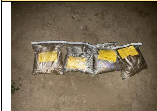
View of Soil samples (left to right order) S2, S1, S3 & S4 from the Depth of 0-2.5m at Project Site.
